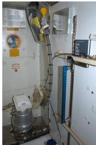
Figure 16. The waste management installed on the ISS, the proposal is to simply modify the size and shape of the feces container but keep the rest of the design
